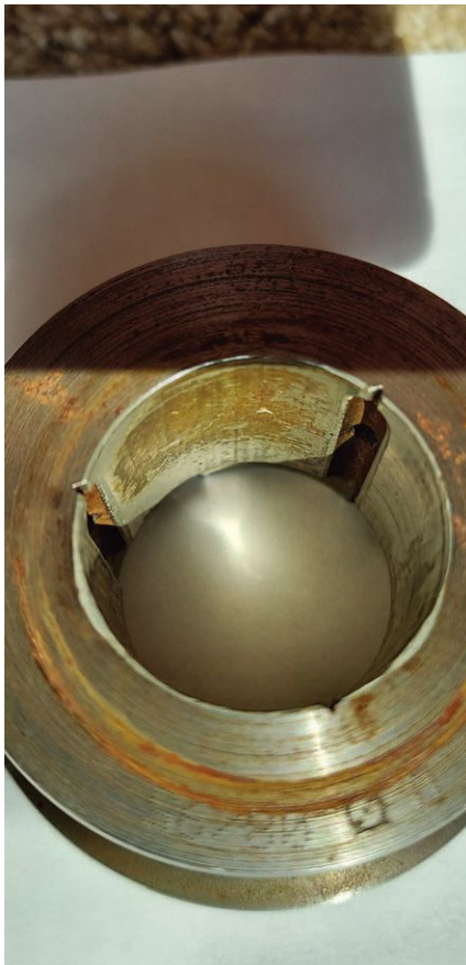
Figure 2. Varnish deposits on a bearing. Figure courtesy of Daryl Beatty.
